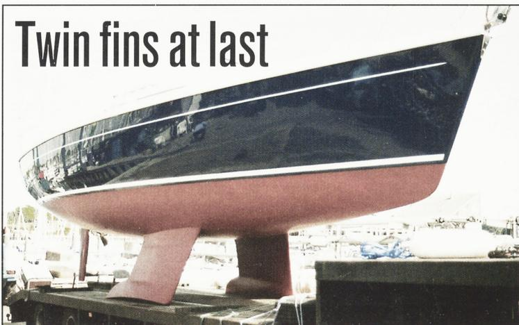
Here's a turnabout for Hunter Boats, builder of a line of capable David Thomas-designed twin keel boats. Although fin keel options have been available for some time, most customers opt to stay with the twins. The reverse has been true for the company's latest boat, the popular Channel 31, which seemed to attract a different breed of owner. Until May only fin-keelers had been launched, but now the first twin-keeler is in the water, complete with Category A (Ocean) classification.
